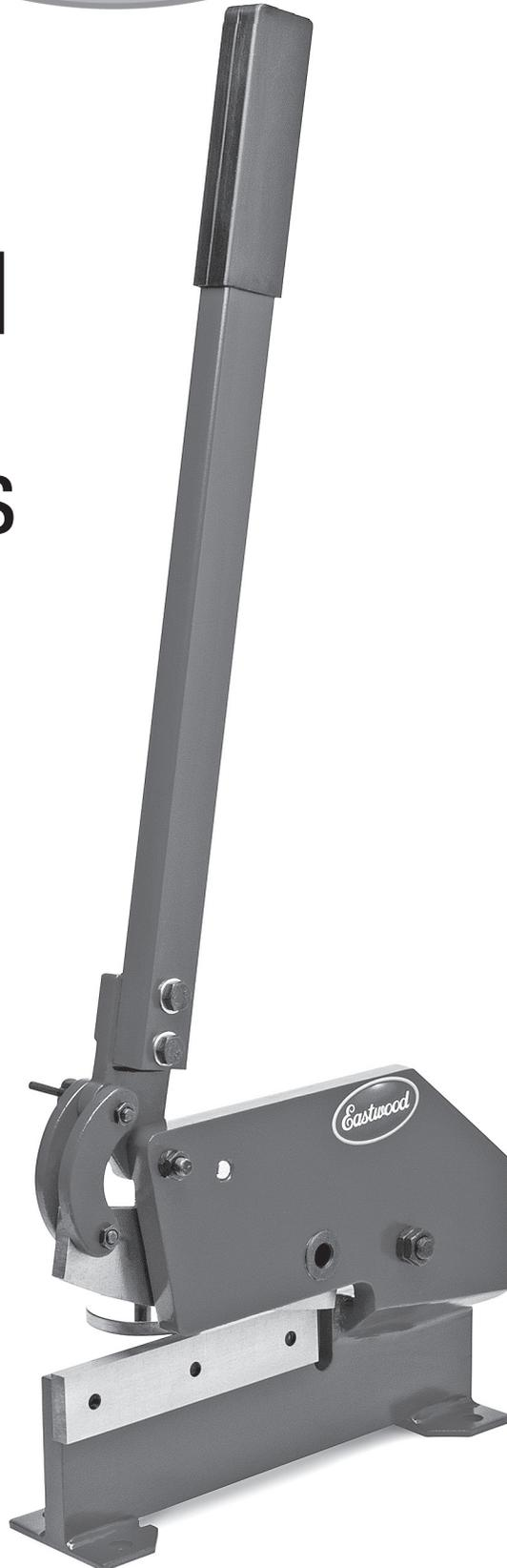
Your **EASTWOOD 8" BENCH SHEAR** for metal cutting is designed for quickly and cleanly cutting mild steel, aluminum and other metals. Torque-amplifying, compound linkage provides low effort and a hardened steel ferrule in the Body, with mating Shear hole in the Blade, allow precision shearing of rod material.
