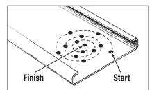
Remove dents with trim hammer, starting at the outside and working inward
