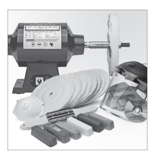
Virtually any metal can be buffed to a mirror-like shine. Aluminum, brass, copper, steel, stainless steel and even many harder plastics can be buffed to a beautiful high-gloss luster using the system of high-quality buffing compounds, wheels and other metal finishing supplies available from Eastwood.
