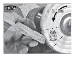
Remove the Compound Bar from the package and holding it firmly, gently apply Compound
