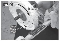
The Buff Rake will also true up an out of round wheel. This is done by first cleaning the wheel
